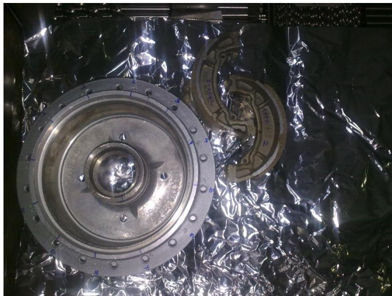
Figure 2 Brake Rotor ready for Cryogenic Treatment
