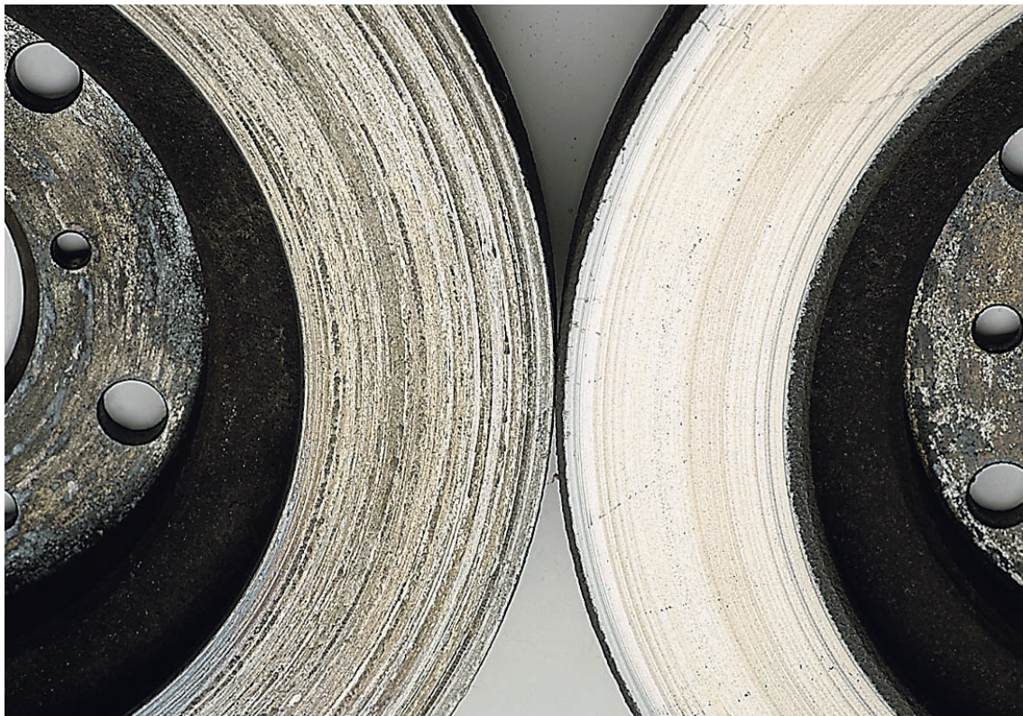
The difference between treated (right) and untreated brake discs after the same amount of hard use
