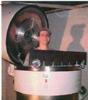
Bill De Felice at Fountainhead Cryogenics stands next to one of Applied Cryogenics' machines. These units operate on liquid nitrogen to get the treated materials down to very cold temperatures.
